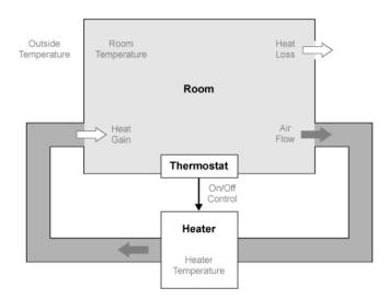
The model for this system includes three components: heater, thermostat, and room.
