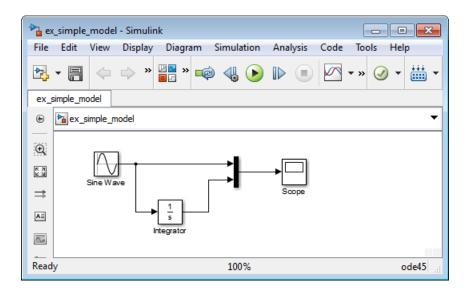
Simulating this model integrates a sine wave signal to a cosine signal and then displays the result, along with the original signal, in a scope window.
