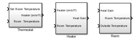
The Room block now has a second input port. Each inport port corresponds to an Inport block in the subsystem.
