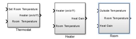
**2** Connect the subsystems as shown.
