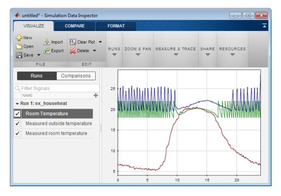
The top signal is the measured inside (room) temperature. The middle signal is the simulated room temperature. The bottom signal is the measured outside temperature.
