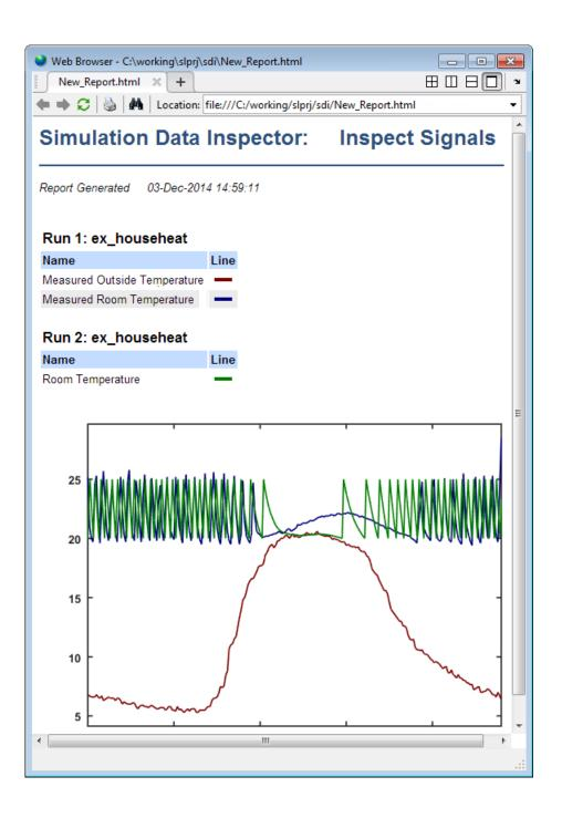
4 In the Simulation Data Inspector, click **Send to Figure**. A plot of the simulated signals opens in a MATLAB figure window.
